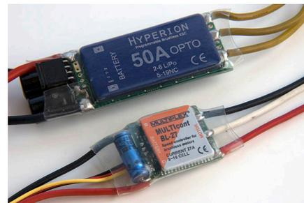
*Two typical brushless motor controllers, 50A unit (top) and 27A unit (bottom)*
