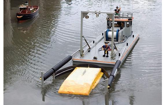
An RC controlled winch and jaws provide the main recovery system. The jaws clamp onto the stalled boat and a life line attached to Argy Bargy's stern bollard is retrieved bringing everything back to shore. The sub-catcher forklift attachment can retrieve submarines, bottles and other debris.
