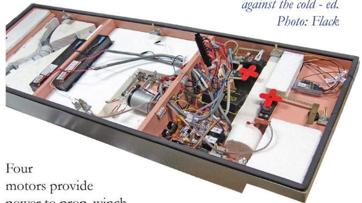
Four motors provide power to prop, winch, water pump and bow thruster. Two 12V batteries supply a 24V speed controller and electrical system which include 6 lights. A four channel 27 MHz radio controls everything. Costs were minimised using recycled materials and commonly available components.
