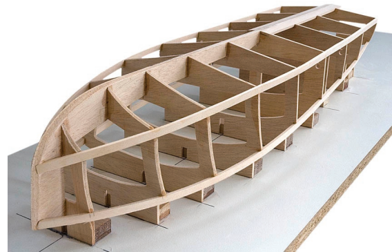
Framework assembly inverted on the building board
