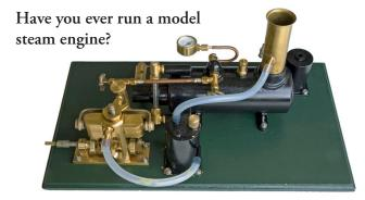
There are all sorts of things you need to do, such as squirt fluids into its various orifices (pure water into the boiler, gas into the gas tank, steam oil into the displacement lubricator, machine oil onto the bearings). Get the levels right. Then you need to light the burner. Use a *long* match!
