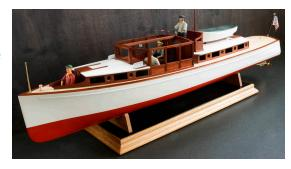
Most of the construction time went into the panelled mahogany cabins, which took far longer to build than the hull. The model has twin shafts and motors and a built-in speaker housing. This currently only provides a horn sound but I may fit a digital engine sound system in due course.
