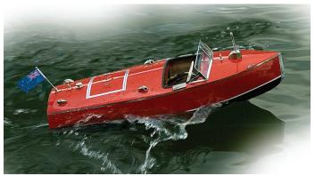
An over-rated drive system consisting of a brushless motor (1400Kv 470W), 40 Amp ESC and 3S Lipo battery were chosen because they would run at low load and stay cool by air convection alone. Weight was kept down by supporting the prop shaft on a nylon bushing inside a strut. The shaft was sealed using a specially made gland containing three 0.1 mm Teflon disks. The motor end of the shaft was mounted in a ball race. Total weight of Boss Drover was 1.342 kg.
